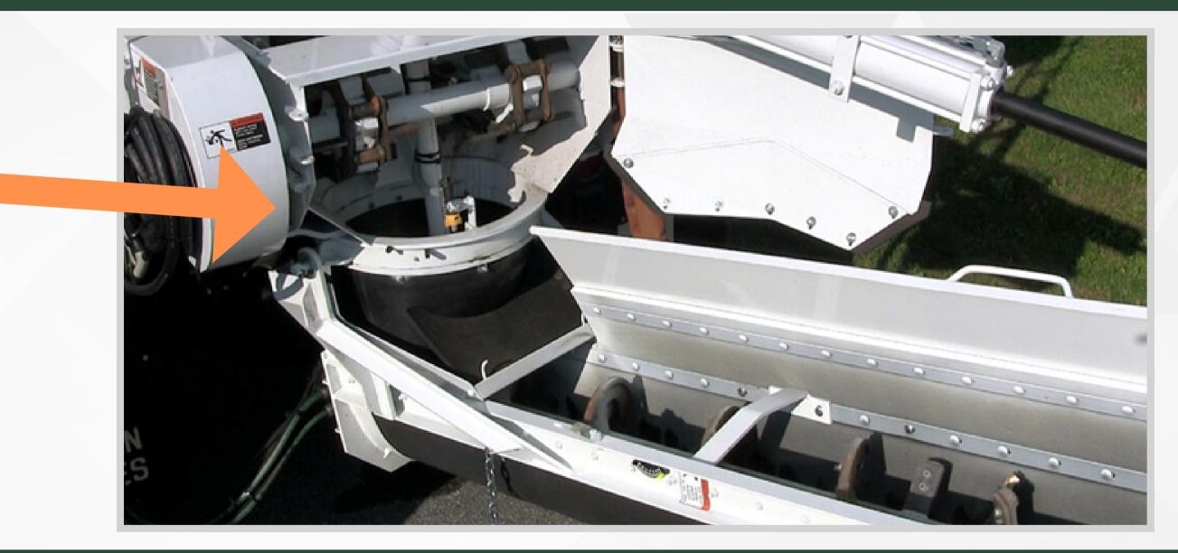
Production averages 60 CY/hr, depending on mix design Ingredients fed continuously during discharge volumetric trucks are known as continuous mixers.
